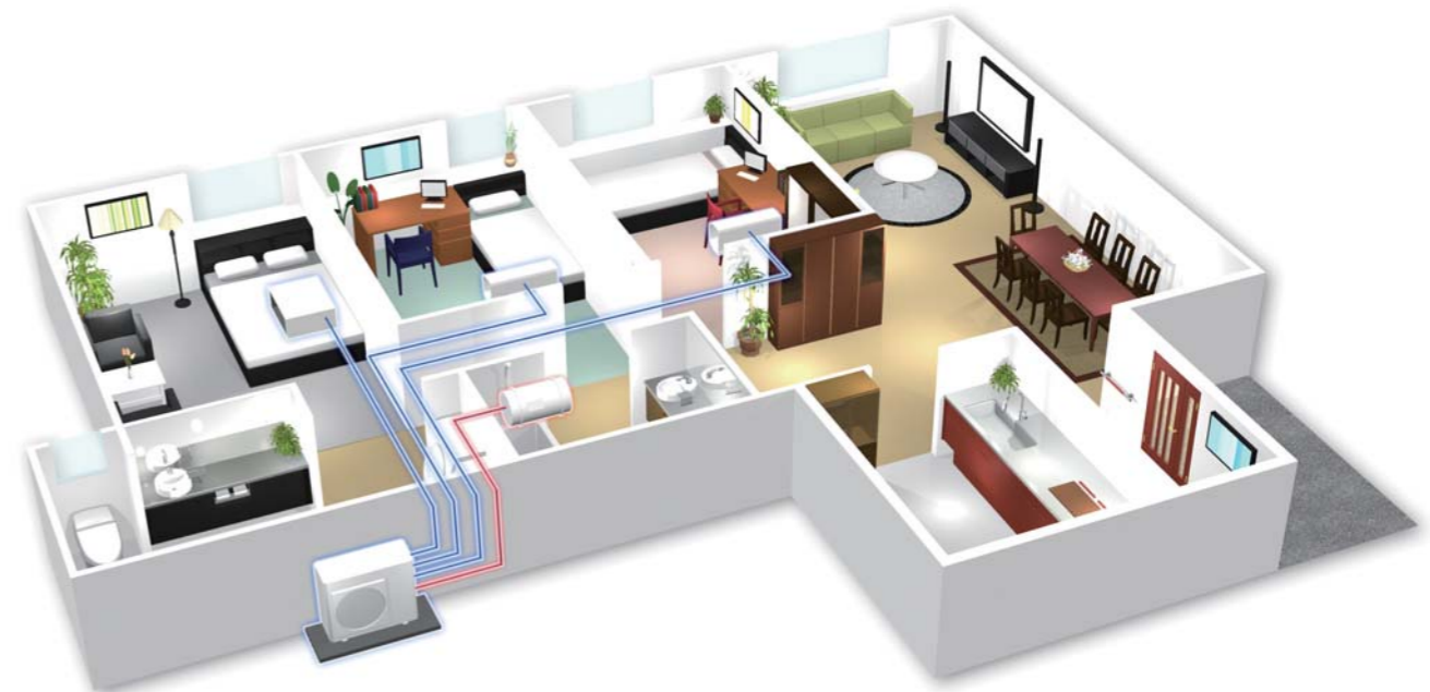
Connect 3 indoor units to a single outdoor unit
