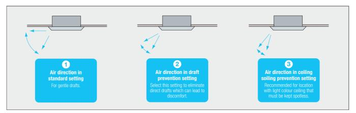
The default setting for air swing pattern is 1. The air swing pattern can be selected through the wireless remote control.
